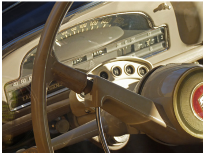
Transfluide gear indicator, unconventional with letters for "normale", "montagne" etc (the operating quadrant lever is to the right, not visible)
