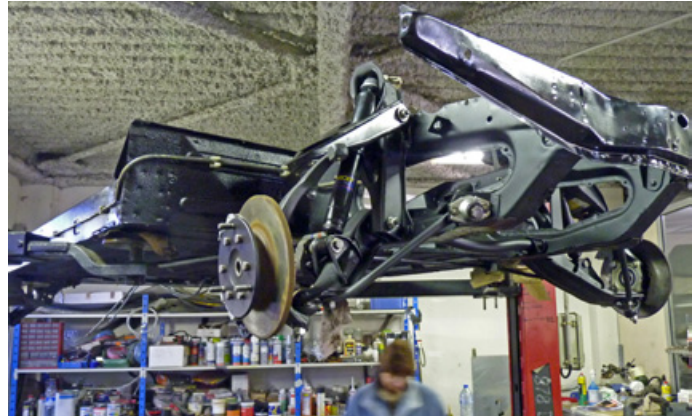
Gazoline workshop with R4 chassis being prepared for a Raid with strengthened front suspension for example
