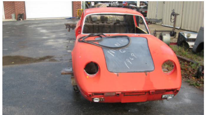
108 body removed and sitting on wooden platform
