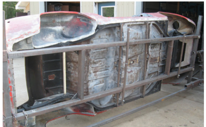
The Glass body being re-attached and final fibre-glassing being doing before the protective coatings will be applied
