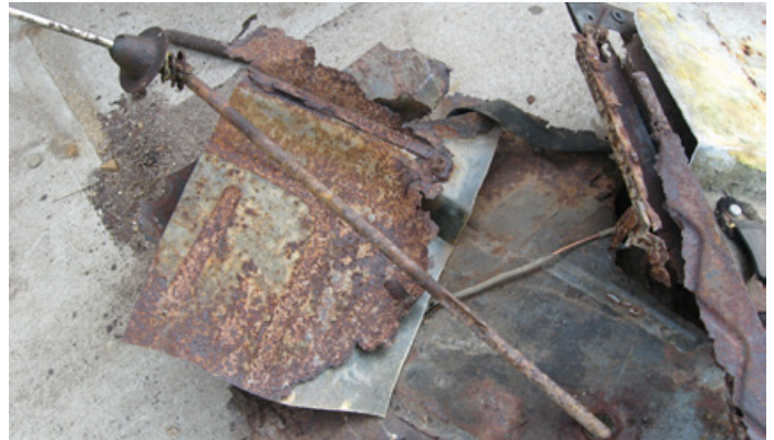
108 rusted out floor pan & frame rails remains
