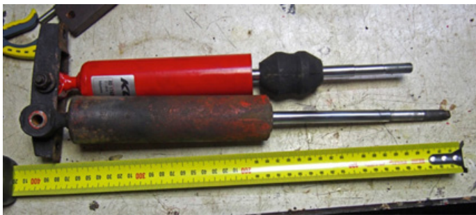
Front Konis, old and new – 35-40 mm shorter for the Gordini
