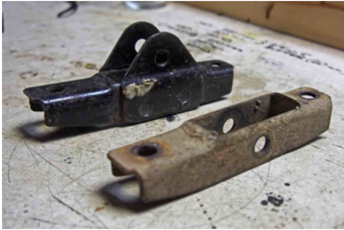
Front shocker mounts new (rear) and old (front)
