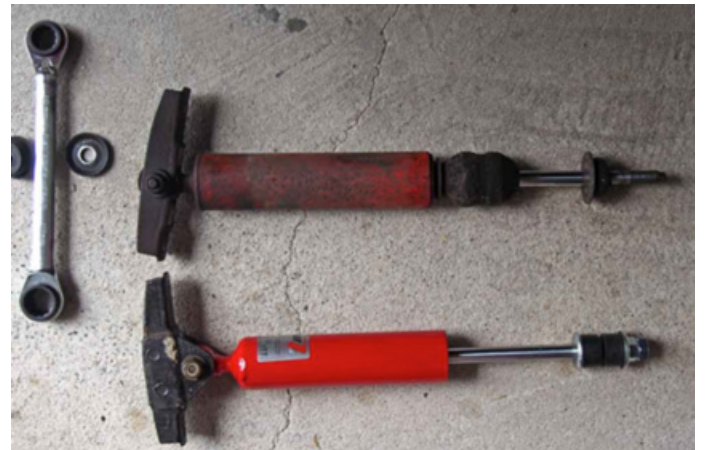
Old Koni 1401 on old mount, new Koni 1743 on extended mount
