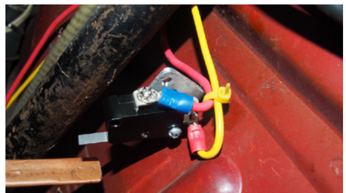
Micro switch mounted on car with inbuilt spring steel actuating blade and wires attached
