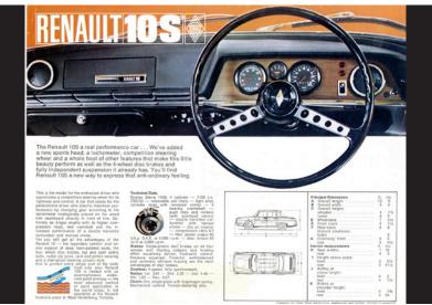
valves and with a dual-choke downdraft Weber carburettor with a manual choke (instead of the usual Solex with automatic choke). The choke was operated with a floor-mounted lever beside the gear lever. The engine developed approximately 60 bhp instead of 48-50 bhp on the standard Renault 10 1100 cc engines which had the 6-port head.
