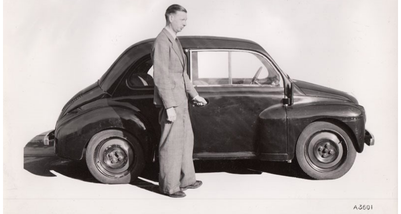
The third or fourth prototype with four doors, sliding windows and spider wheels. ©Renault Communication
