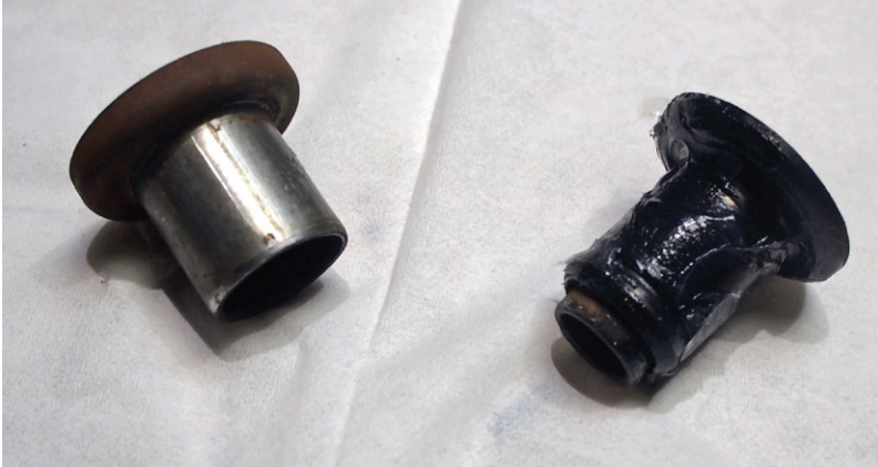
Fluidbloc bush relubricated with silicone grease prior to re-assembly)
