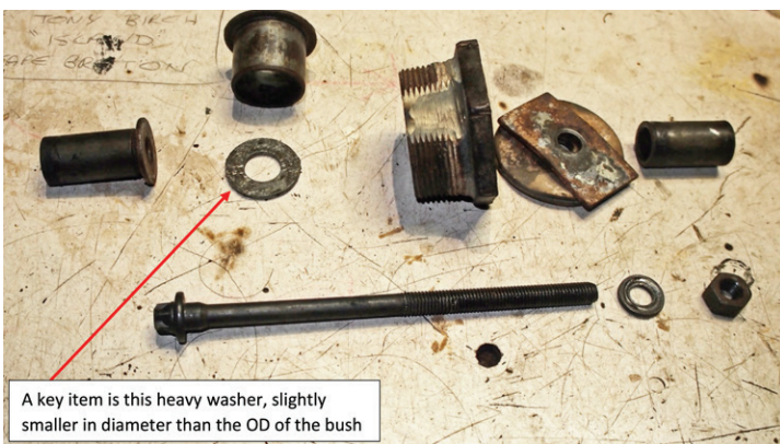
Simple components of tool to pull Silentbloc bush out of lower R8 wishbone
