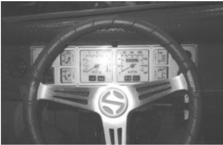
Photo above: R5 switches, speedo, fuel gauge and voltmeter with new d.i.g. faces. R5 instrument lamps, windshield wiper mechanism, and heater. R5 seat belts.
