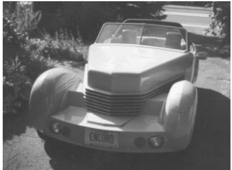
Car is Cord-inspired. Renault R5 seats, mirror. Windshield frame cut down from R5 door window frames.
