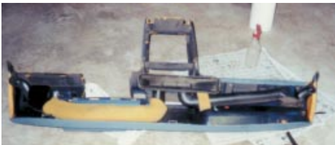
Dash with one of the insulated ducts in place.
