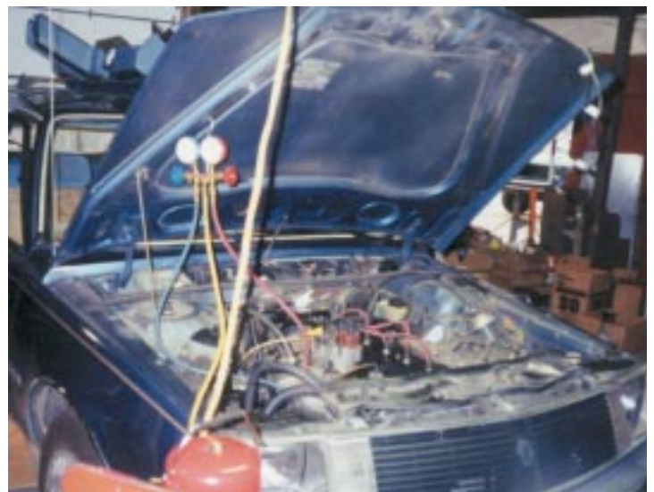
Pumping down the system and loading freon. Note vacuum reservoir just to right of coolant bottle.
