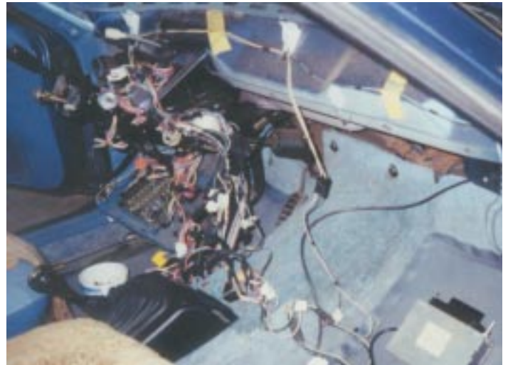
Everything taken out and ready for A/C installation.
