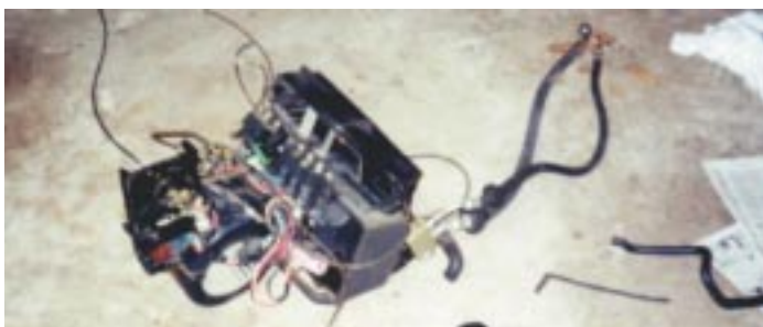
A/C unit w/ hoses, wiring. Note 6 relays at wire plugins.
