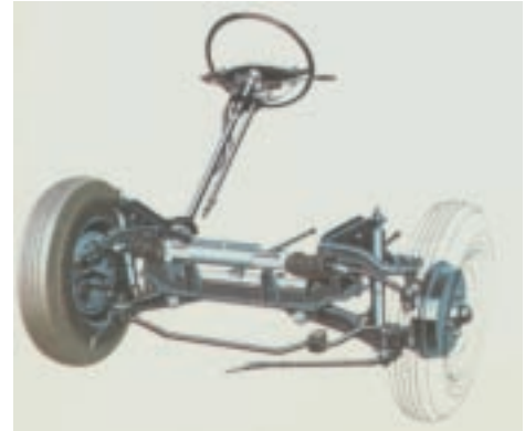
Right: Contessa 1300 front suspension and steering.
