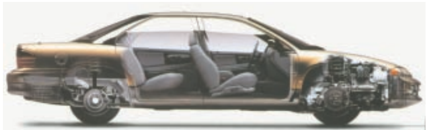
Above: Dodge Intrepid showing longitudinal V6 ahead of front axle and strut front suspension inspired by R25/Premier. From Dodge Division.
