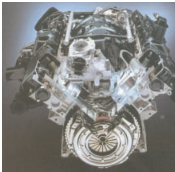
Left: Renault 25 V6 injected, 2664cc, 144bhp.
