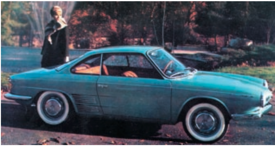
Left: Hino Contessa 900 Sprint by Michelotti. 893cc OHV, 45hp @ 5000 rpm, Weber carb, 3 or 4 speed transmissions, front disc brakes. Below: front and rear views, interior. Door sill reads "Hino- Michelotti." Hino Publicity.
