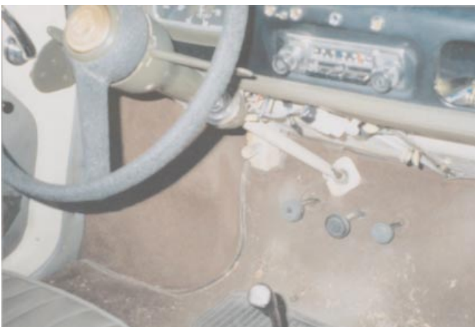
New speedo decal, multiple wire jack, radiator blind control, R10 shifter stick, warning lights above radio.
