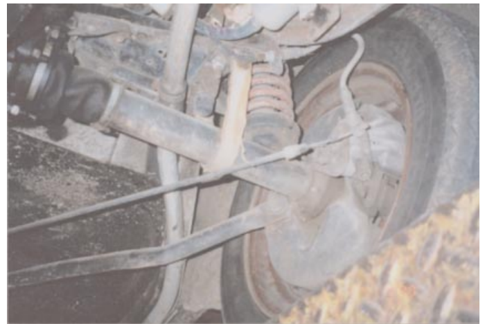
Electric high pressure fuel pump top, conduit water line, hand brake cable tweaking rear caliper, radius rod bolted to backing plate.
