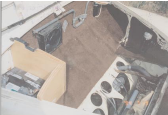
Above: temperature control blind pulled up. Below: Heater muffin-fan, battery box sealed off from heater air, carpeted trunk for insulation.
