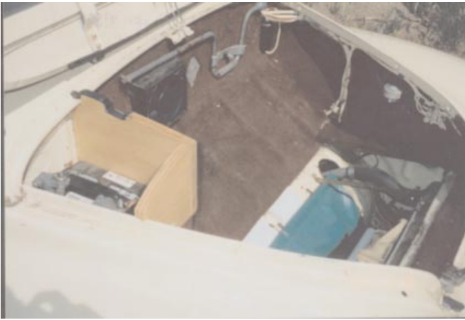
Above: temperature control blind pulled up. Below: Heater muffin-fan, battery box sealed off from heater air, carpeted trunk for insulation.
