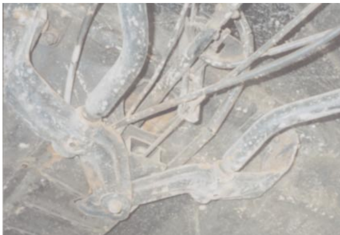
Controls; swing arm handbrake connection, radius rod addition, shifter rod adjustment (2 through bolts), battery cable going up front, speedo clutch & throttle cable, water pipe at bottom corner.
