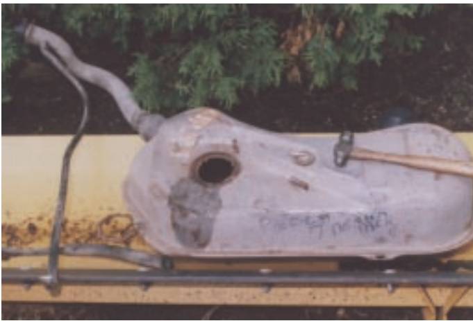
This was the old fuel tank, Full of shellac and rust. Not even good enough to boil out. Strangely, this was not an original '86 tank, but one from 1984. It had been replaced for some reason, early on.
