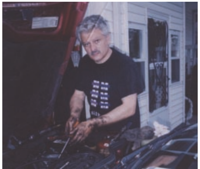
Jerry Vella replacing the timing belt and idlers on Jesse Patton's '85 Alliance convertible. It was time after 58,000 miles.
