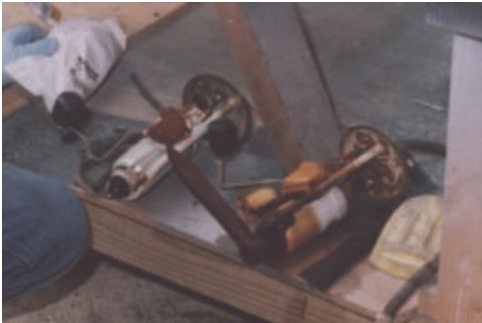
Johnny Schuler an old-time Renault mechanic looks over the old fuel pump on the right which is an '86 Bosch with the low fuel light sensor. Both the sender unit and the pump were rusted and useless. The '85 Bosch pump on the left will be used in its place.
