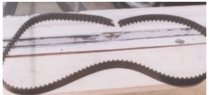
No mistaking a broken timing belt. Always replace it every 60,000 miles, and spin both idlers to make sure they are free and easy.
