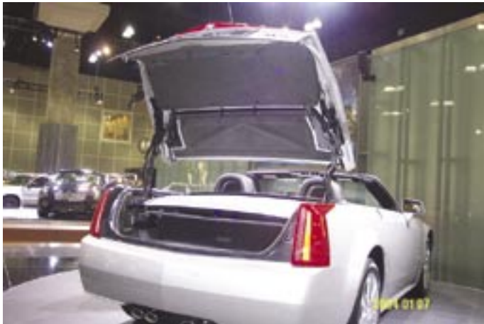
Above: Cadillac XLR showing the retractable top stowed. Below: Mégane Convertible Coupe with its top operation. Right top to bottom: new Mercedes SL and view of the interior with the top lowered; Lexus SC430; Peugeot 206cc, with top operation.
