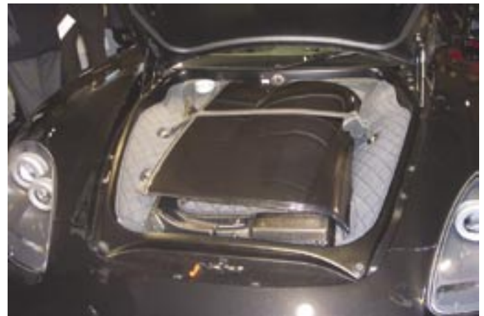
Above: Porsche Carrera GT showing stowage of the removable hard top halves in the limited front trunk space.
