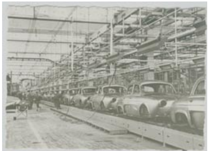
11. (below) Pierre Lefaucheur at Flins. Assembly line for bodies-in-white before painting. The Pierre Lefaucheur factory is considered one of the most modern in Europe.
