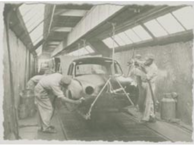
12. (above) Pierre Lefauchaux at Flins. One of the paint booths. Renault uses 20 metric tonnes of paint daily, produced by its factory at Mans.
