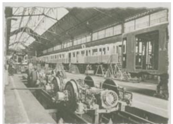
17. (below) Choisy-le-Roi factory. Ironworks division. Construction of Métro subway cars which use tires. Renault also builds turbine locomotives and tanks.
