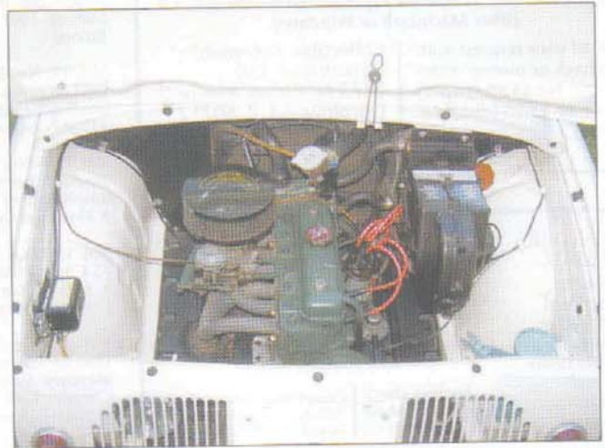
1-5. The Dauphine line expanded in the early Sixties to include better-equipped luxury models and, in 1962, the limited-edition rally-bred R1093 model. The "Ventoux" inline four in the R1093 generated a hefty—by Dauphine standards—55 horsepower. Regardless of model, Dauphines could carry seven cubic feet of luggage beneath the front-hinged lid of their cargo bay. This well-lighted R1093 was originally sold in Sweden and made its way to Mexico in 1999. 6, 7. The '62 base-model Dauphine was improved through the adoption of a fully synchronized three-speed transmission. As always, the rear half of the back-door windows slid forward for ventilation. (Owner, both cars: Miguel Garza Hoth)
