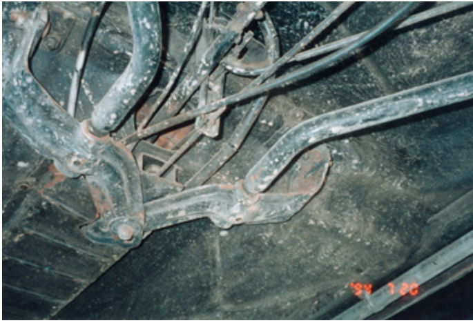
Controls: swing arm hand brake connection, radius rod addition, shifter rod adjustment (2 thru bolts), battery cable going up front, speedo, clutch & throttle cable, water pipe at bottom corner.
