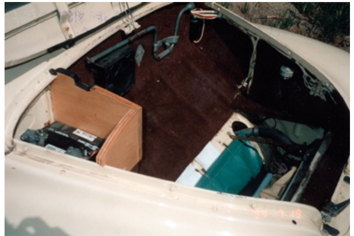
Top-heater muffin fan, battery box sealed off from heater, carpeted trunk for insulation.
