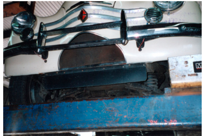
Radiator behind modified bumper & missing chin, air dam hangs below.
