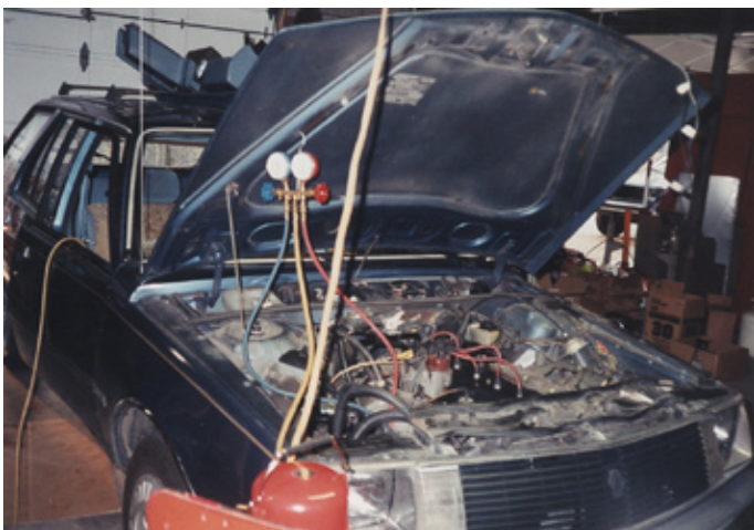
Pumping down the system and loading freo. Note vacuum reservoir just to right of coolant bottle
