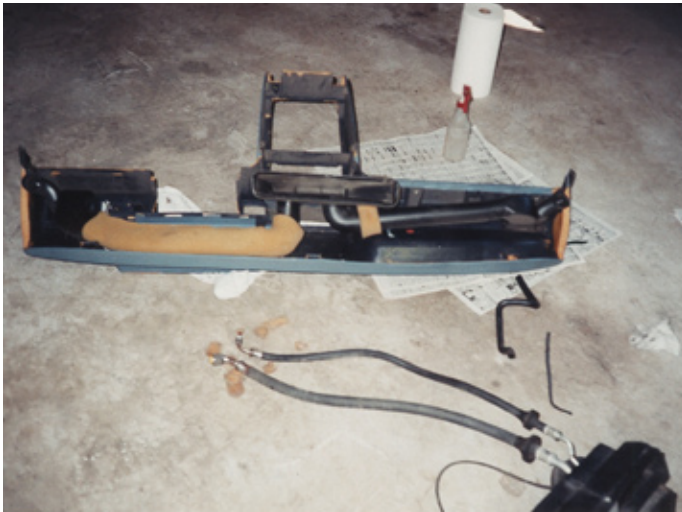
Dashboard with one of the insulated ducts in place
