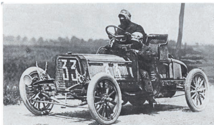
Barbarou on a Benz, with headlight brackets drilled to save precious weight.
