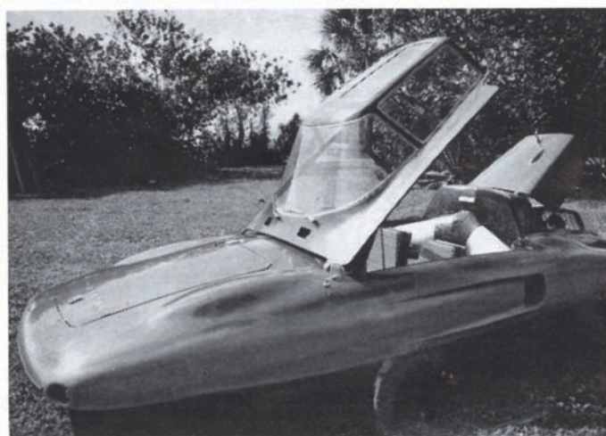
Front lid, canopy and engine cover are hinged at front.
