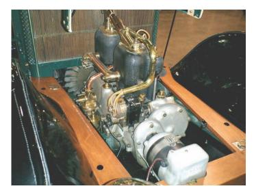
pointed out to me that the fly wheel had vanes on it which served as a fan to draw air into the engine compartment and probably through the enclosed portion of the radiator. It follows the same principle as fans on modern radiators.
