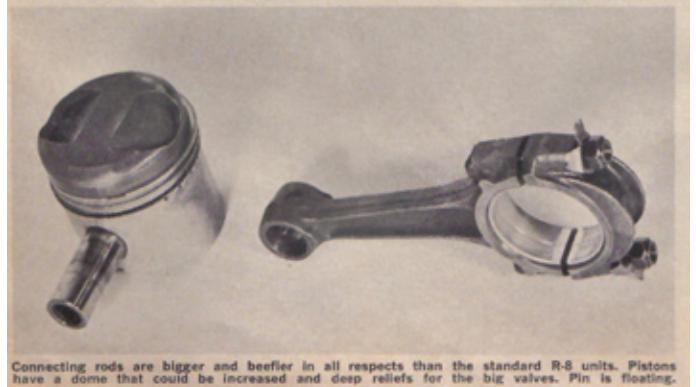
Connecting rods are bigger and beefier in all respects than the standard R-8 units. Pistons have a dome that could be increased and deep reliefs for the big valves. Pin is floating.
