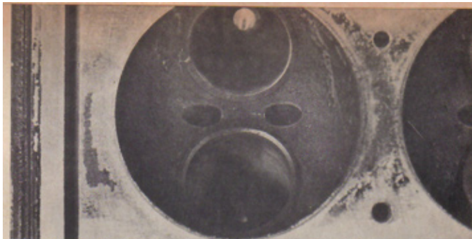
Detail of combustion chamber in the Gordini head shows the relatively large valve seats and the cartridge-fire flame passages. Ports are direct, large and well-shaped for good flow.
