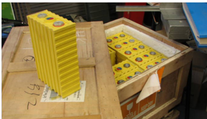
This is a 3.2 Volt, 90Ahr lithium cell. It weighs just 3 kg. I bought 38 of 'em:
