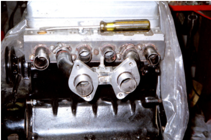
Start of custom intake/exhaust manifold
